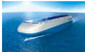
ISHIN-I Hybrid car carrier utilizing renewable energy
