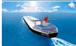
ISHIN-III Large ore carrier with high-efficiency waste heat energy recovery system
