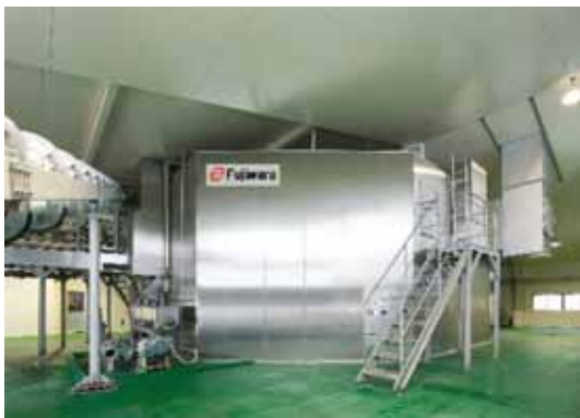
Rotary type automatic Koji making equipment
