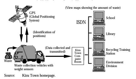
Mechanism of next-generation GIS model operation
