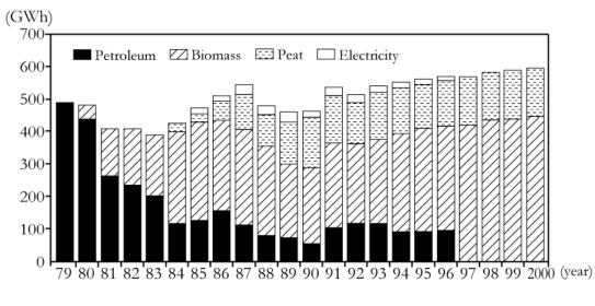
Figure 5: Shift of Energy Source in Växjö (1979-2000)
